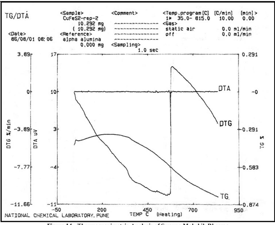
Figure 14 - Thermogravimetric Analysis of Swarna Makshik Bhasma
