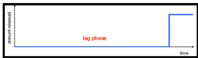
Figure 5: Expected behavior and release profile of swellable/erodible reservoir systems for oral pulsatile delivery
